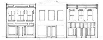
The new building at the center respects the traditional division of the façade into upper and lower sections and maintains the traditional arrangement of storefront and upper elements.
