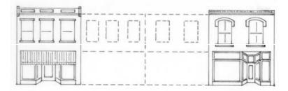
These new buildings respect the existing height pattern and horizontal & vertical window alignment.
