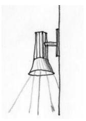
Simple metal extended-arm fixtures are appropriate for illuminating commercial buildings and signs.
