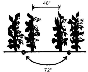
**Figure 13.** One trickle line for every two rows.
